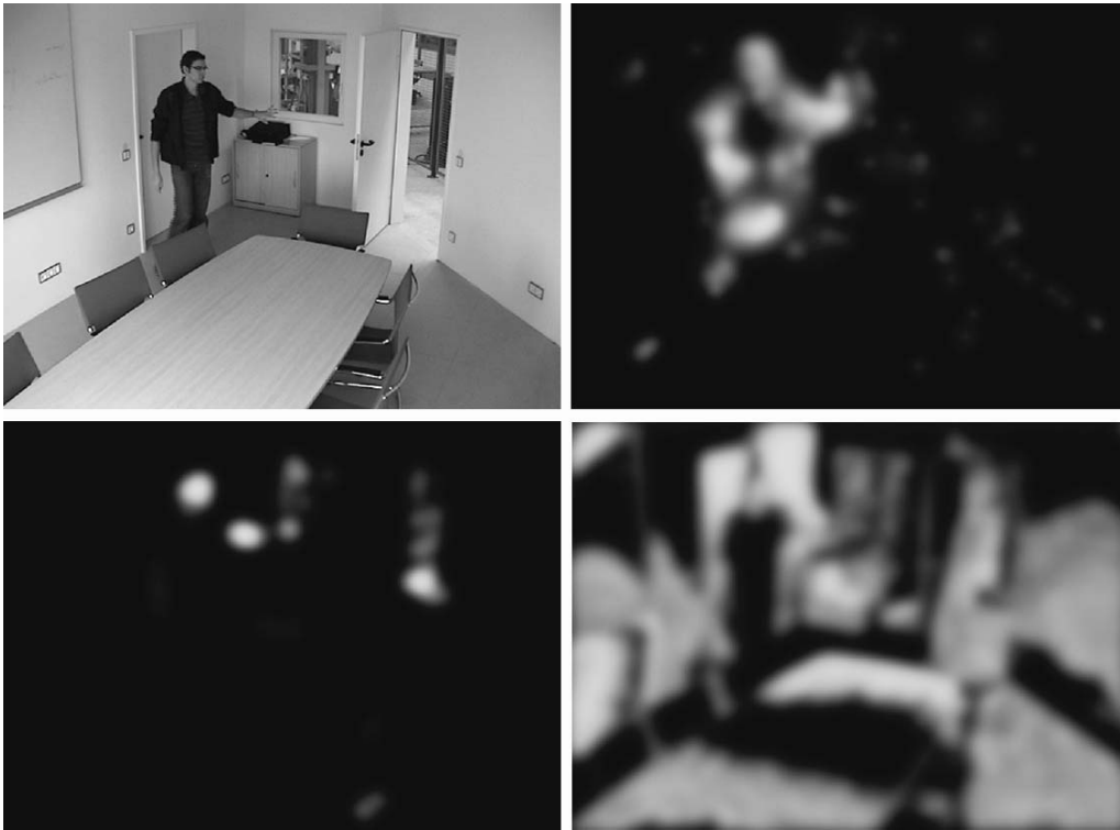
Fig. 4. Examples for saliency maps. From left to right, top to bottom: original image, SIFT saliency, skin saliency ( L^*a^*b^* classifier), skin saliency (nRG classifier).
