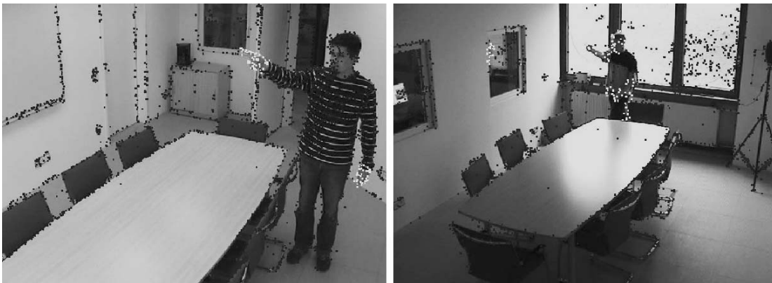
Fig. 3. Examples for SIFT based hand detection results. Sift key points are depicted by squares, white squares represent positives, black squares are negatives. Left: very good detection, the hands are identified correctly and almost all false positives are discarded. Right: here, the filtering algorithm fails because the false positives form large clusters.
